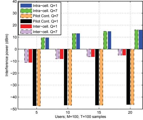
Fig. 3: Interference components in mmWave systems using Q=1 and 7.
