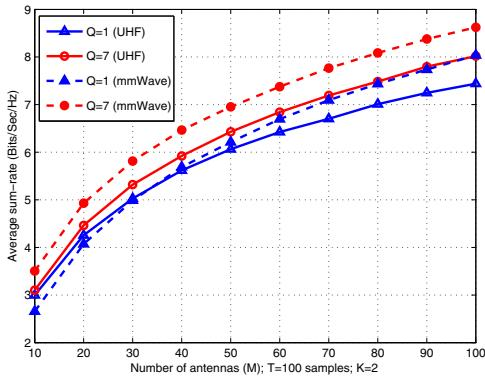
Fig. 6: Average throughput versus number of BS antennas at  $K=2$ .
