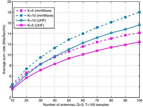
Fig. 5: Average throughput versus number of BS antennas at  $Q=3$ .
