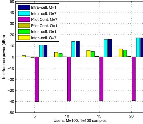
Fig. 2: Interference components in UHF systems using Q=1 and 7.
